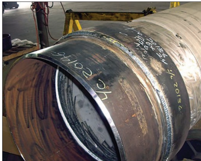
A dielectric coupler used to insulate connection between dissimilar metals, reducing corrosion.
