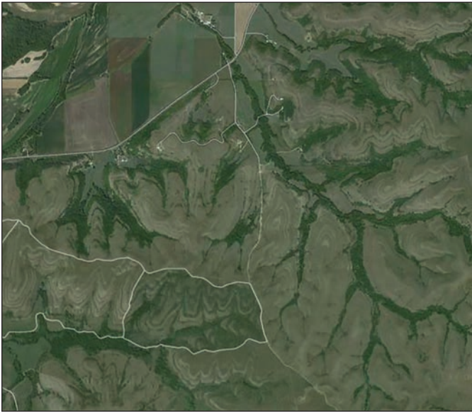
Satellite image of the Konza Prairie in north central Kansas. Images such as these can be used to help identify watershed boundaries and assist with delineation of the source water protection area for a well and its area of recharge.
