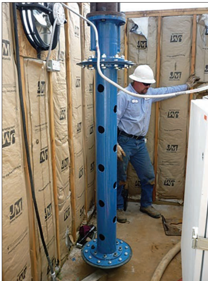
An isolation tool used as a double disk surge block to aid development efforts. The tool allows for a combination of air lifting and swabbing while pumping or injecting chemicals.
