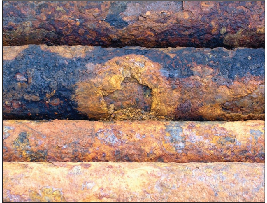
The nail test showing exposure for one year. The test is from two separate aquifers both with a positive saturation index.
