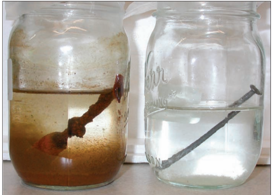
The nail test showing exposure for one year. The test is from two separate aquifers both with a positive saturation index.
